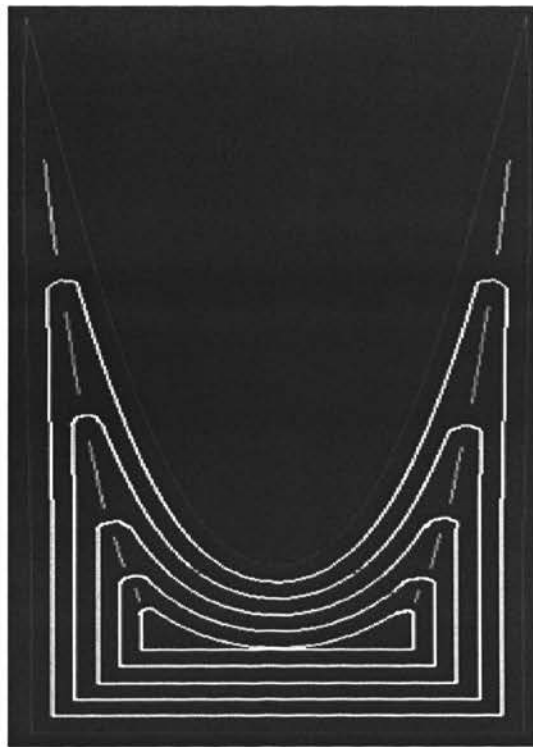
Figure 5.7 Offset Example after Path Adjustment
