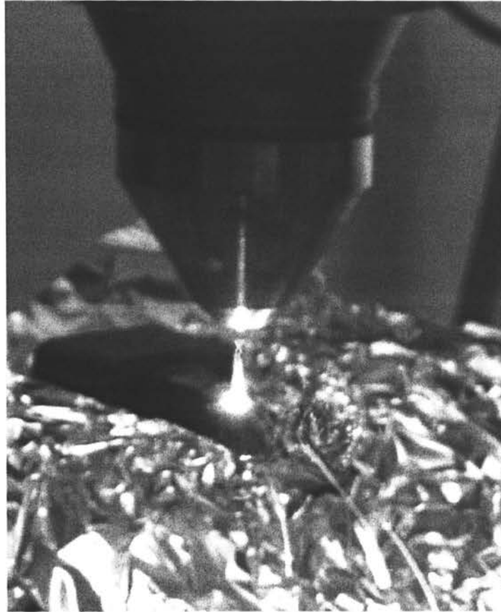
Figure 3.2 LAMP Deposition Process using the Laser Beam
